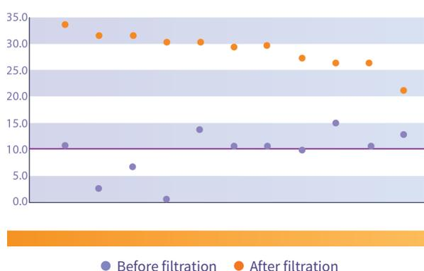
Arsenic concentration (ppb) at the Yacango Treatment Plant before and after the filter
