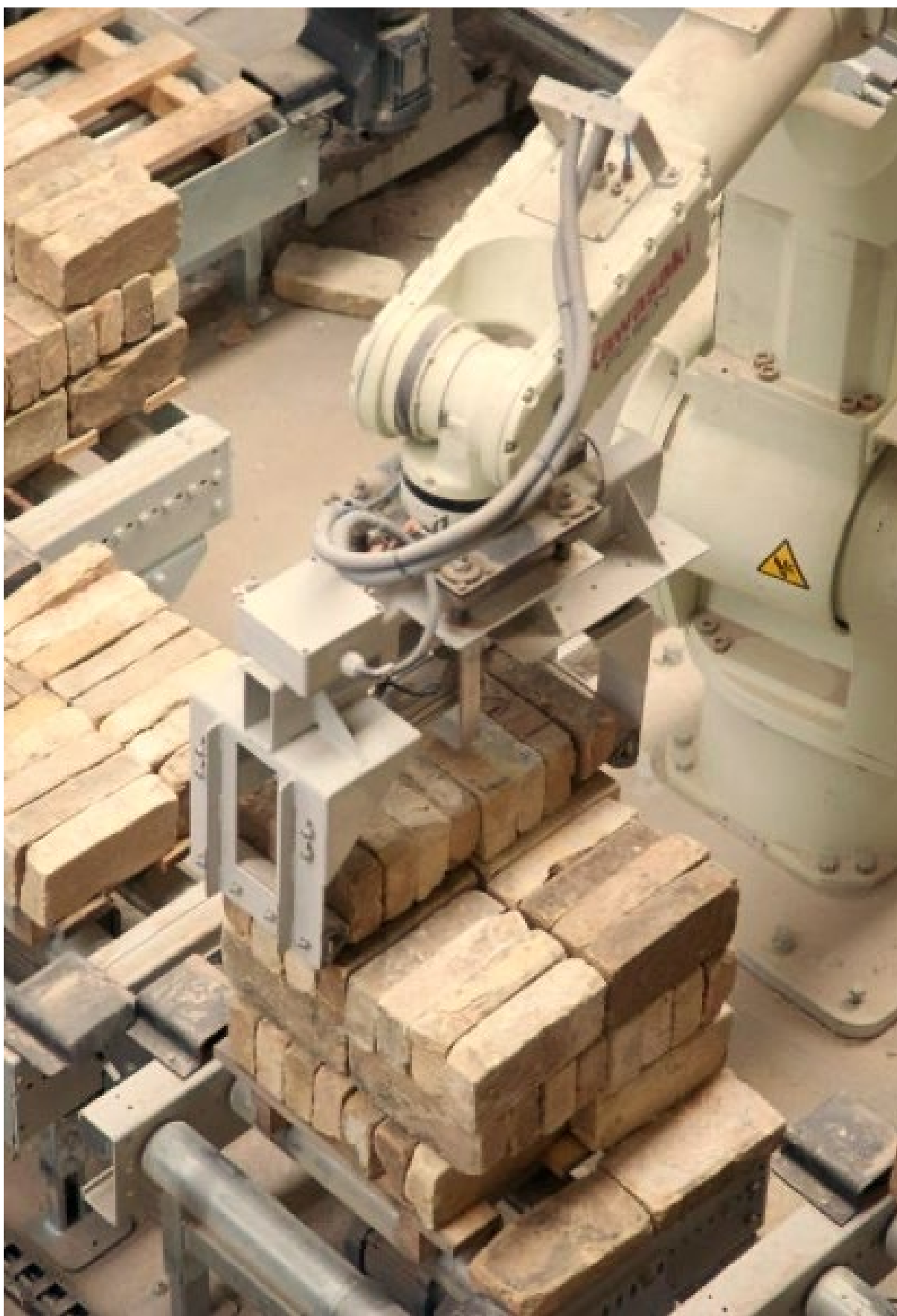
Robotized brick handling in Scandinavia (Web image 11)
