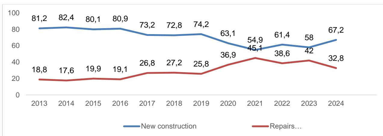
During 2013-2016, Ukraine maintained a consistently high share of new construction (including reconstruction), exceeding 80%. Starting in 2017, a gradual change in structure was observed: the share of new construction began to decline, while the volume of repair work increased. The most noticeable reduction in the share of new construction occurred in 2020–2021, to 63.1% and 54.9%, respectively. In 2021, it reached a minimum of 45.1%, accompanied by a peak in repair work of 36.9%.
