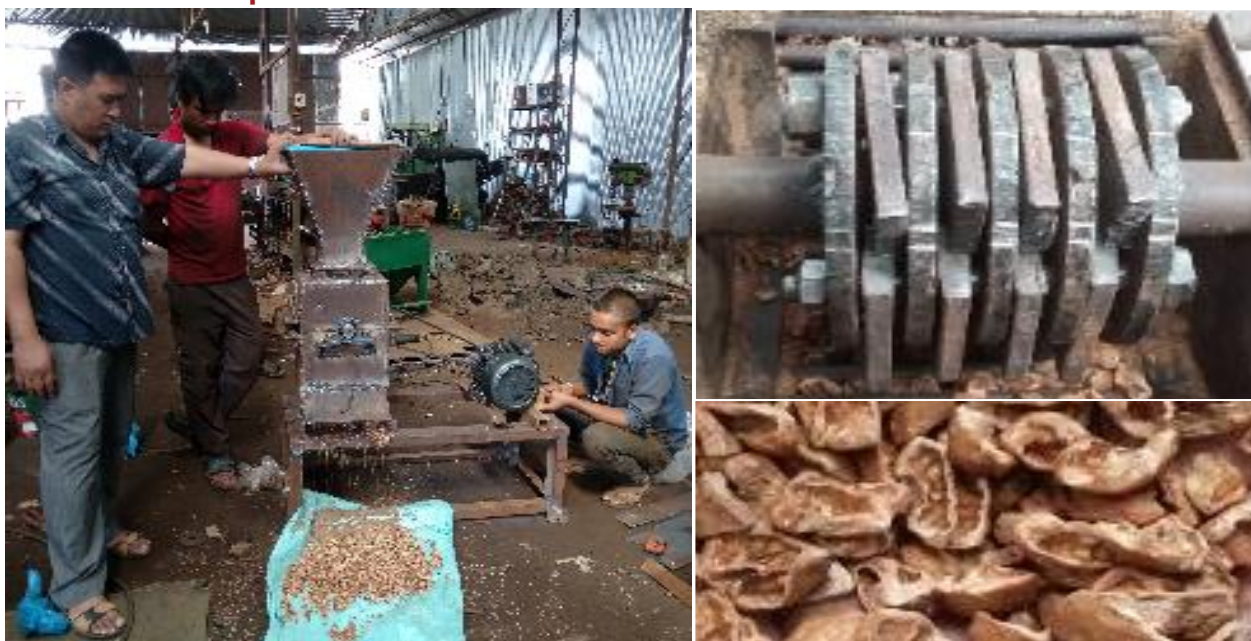
Picture: Testing the performance of hammer based walnut crushing at Bhaktapur workshop, 2018
