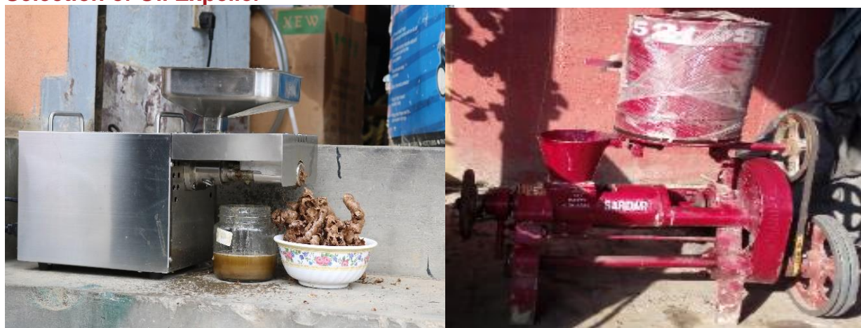
Picture: Korean oil expeller for home use(left) & Indian Oil expeller for commercial purpose (right)
